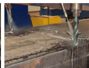
09_Make welding hole
